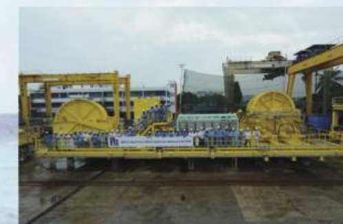
550 ton Riser Pull-in Winch System for P66
