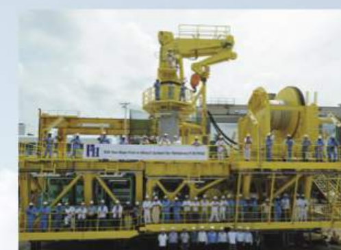
550 ton Riser Pull-in Winch System for P74
